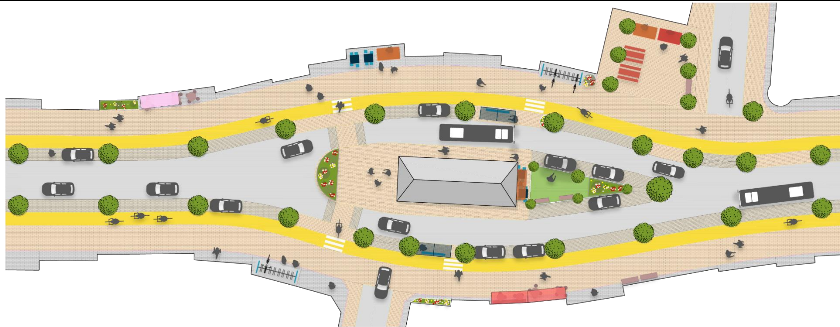
Figure 4-10: Typical Layout Diagram - Type 2(a) - High Streets - Arterial High Activity
