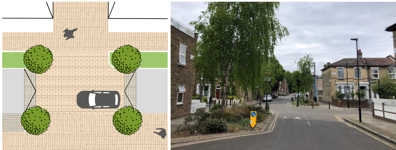
Figure 5-3: L: Diagram showing raised plateau at junctions slowing traffic and providing level crossing for pedestrians (Credit: Create Streets) R: Retrofitted to historic streets in Highbury, London , note the excellent use of trees and greenery to narrow the carriageway and retained kerb lines (Credit – Create Streets)
